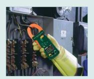
Large jaw size for high current measurements
