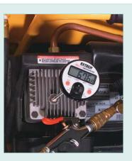
Flat surface stem thermometer ideal for measuring high temperature on motors and other flat surface areas including grills.
