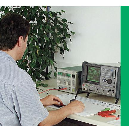
Built-in spectrum analyzer
