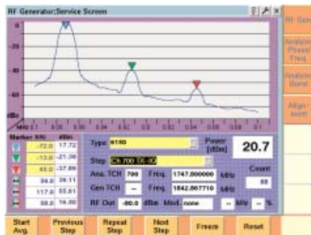
Alignment screen: Combining generator, analyzer and spectrum analyzer functionality.
