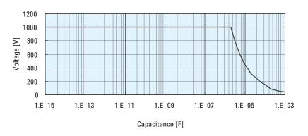
Figure 8. Maximum discharge withstand voltage
