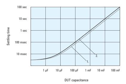
Figure 11. DC bias settling time
