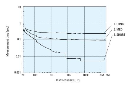
Figure 9. Measurement time (DC bias: OFF)
