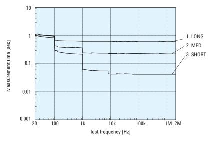
Figure 10. Measurement time (DC bias: OFF, Option 005)
