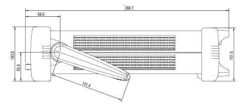
Figure 6. Dimensions (side view, with handle and bumper, in millimeters, nominal)
