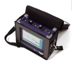
MTS/T-BERD 8000 platform with OTDR and OFI modules
