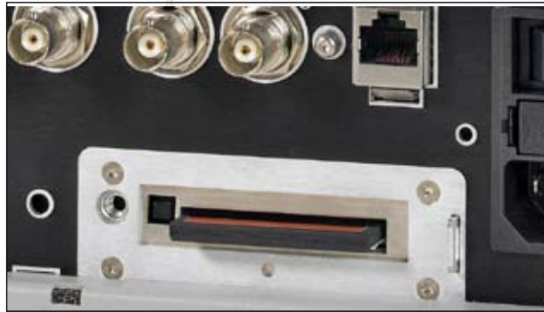
CompactFlash™ Card ejector on instrument rear side
